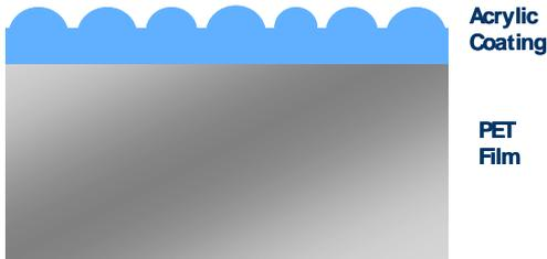
Figure 3. Coated diffuser.
