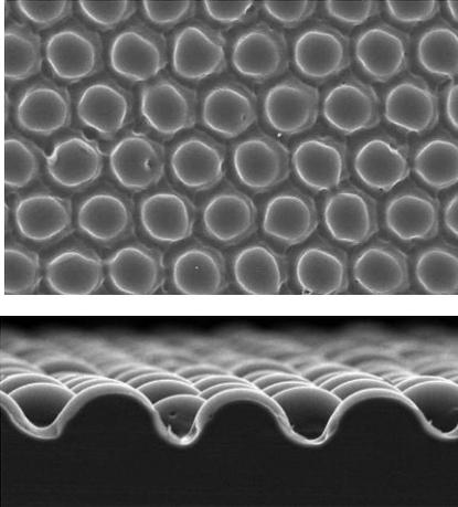
Figure 7. SEM of Basic Lens Diffuser Film.
