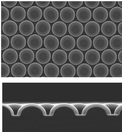
Figure 8. SEM of High-Gain Diffuser Film.
