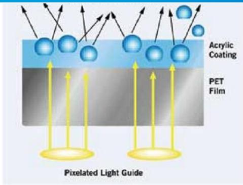
Figure 2. Bead-filled coated diffuser.
