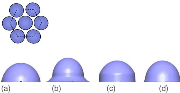
Figure 5. Micro-lens contours used for simulations.
