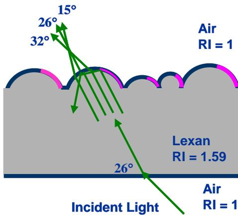
Figure 4. Ray tracing approach.
