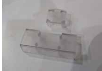
Pieces separated by scoring and bending along groove
